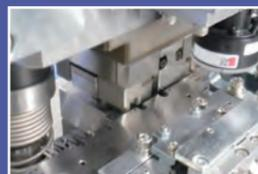
Stamping process for HDD suspensions using high-precision dies
