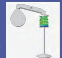
Computer simulation to visualize the behavior of valve springs when driven at high speeds
