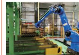
Automatic conveyance and electric sintering treatment by robots for realizing labor and energy savings (Suspension Spring Business)
