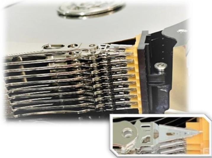
Suspensions for HDD are unique spring products, holding read-write head in Hard Disk Drive devices.
