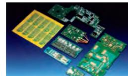
Metal base printed wiring boards
